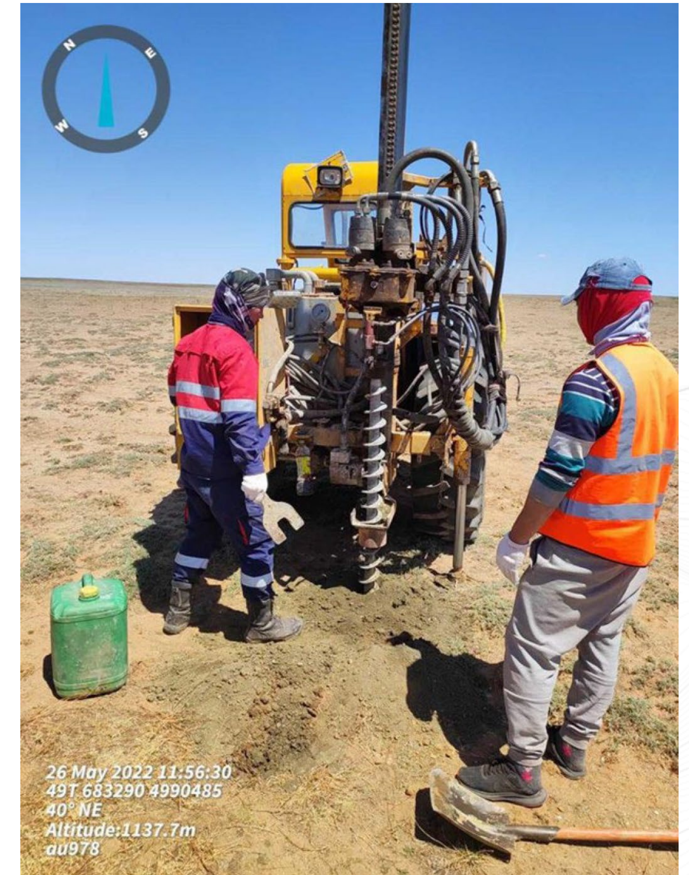
Figure 2: Auger Geochemical Drilling Rigs at the Victory Discovery.
